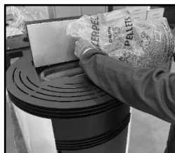
Figure 12 – Refilling the pellet tank
