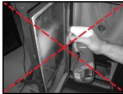
Figure 13 - Incorrect glass cleaning
