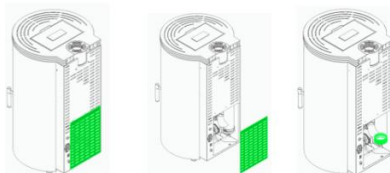
Figure 21 - Cleaning the "T" inspection
