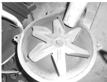
Figure 20 - a) Aspirate the extractor shell; b) Vacuum the pump
