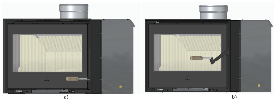
Figure 19 - a) Correct position of the key, b) Door opening movement
