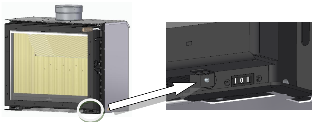
Figure 51 – Door handle adjustment, micro-switch actuation
